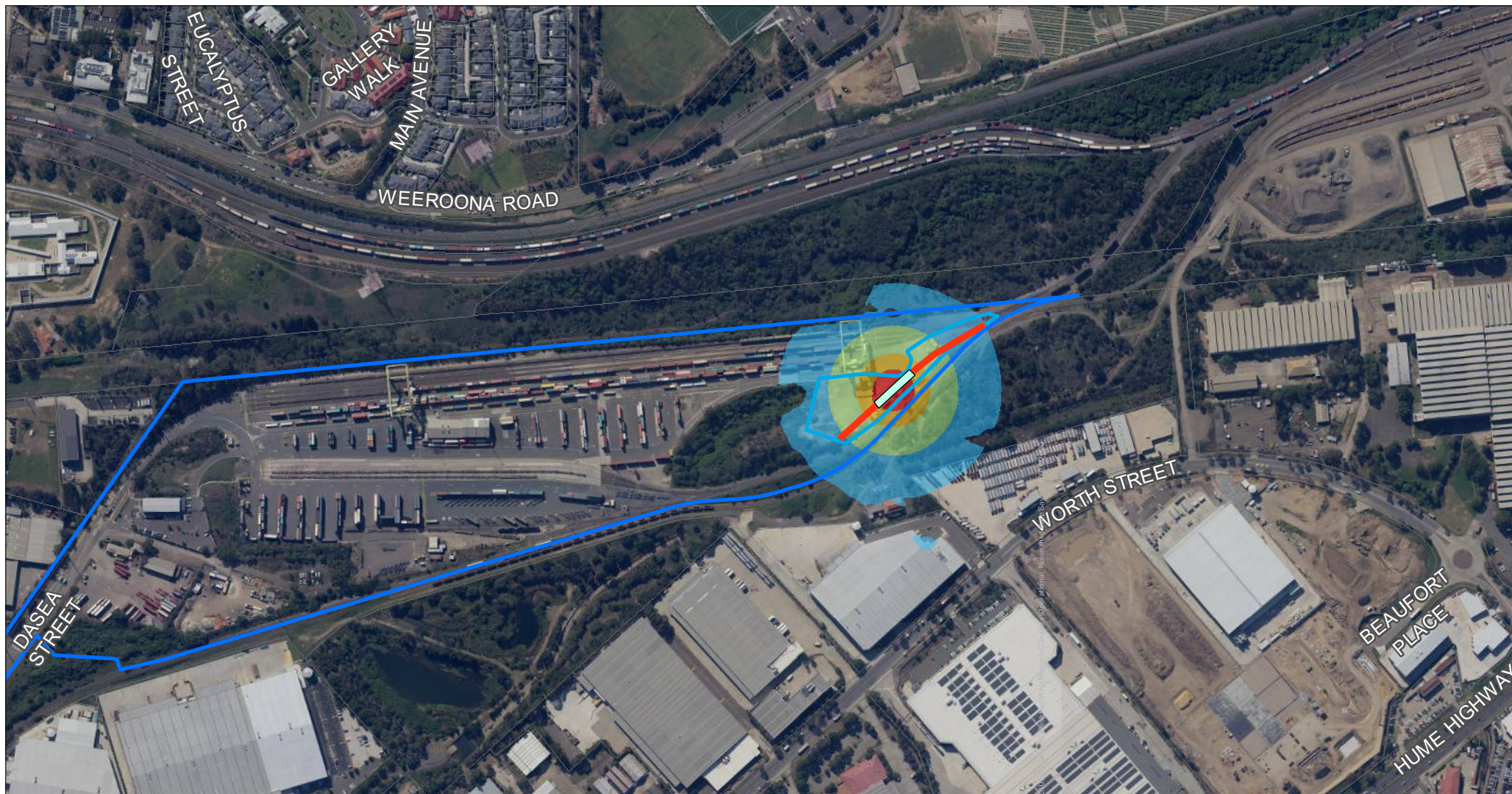
Locomotive Provisioning Centre - Maximum Noise Levels - Neutral Conditions
