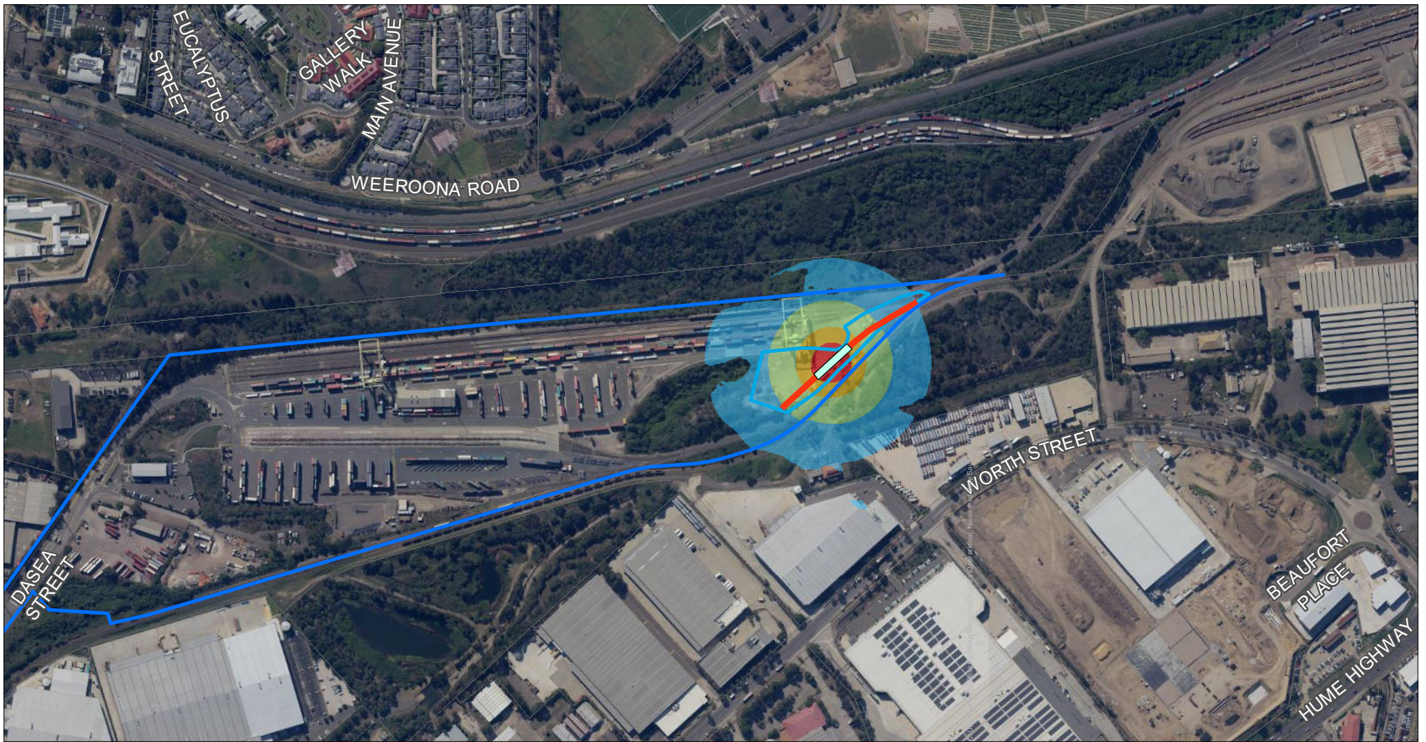
Locomotive Provisioning Centre - Maximum Noise Levels - Temperature Inversion
